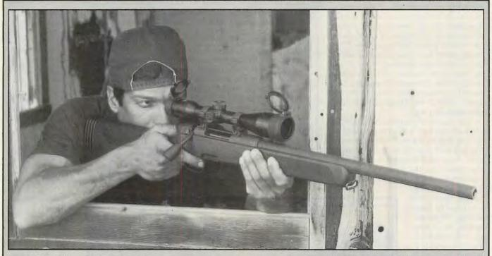
Steyr's SSG-PIIK sniper rifle with a 20-inch barrel and equipped with the excellent Hensoldt 10X scope with 3/4-minute Mil Dot reticle pattern provides a highly accurate, yet compact envelope especially suited to law-enforcement tactical teams deploying in crowded urban environments.
